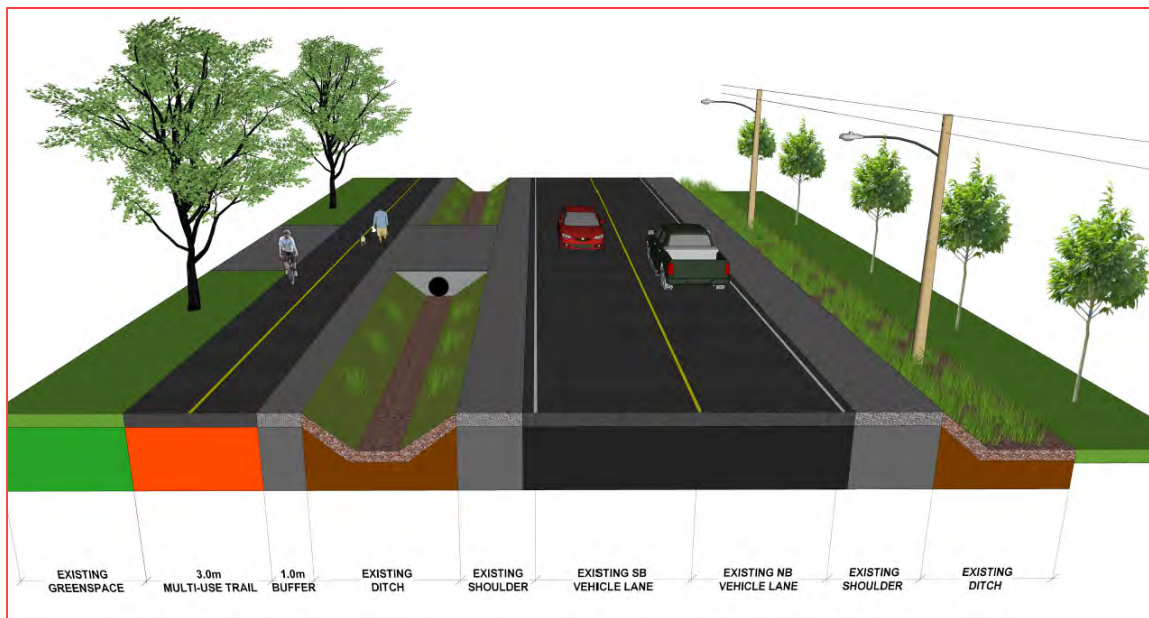
Figure 6-2: Proposed Lucasville Road Cross Section with existing ditch looking north
