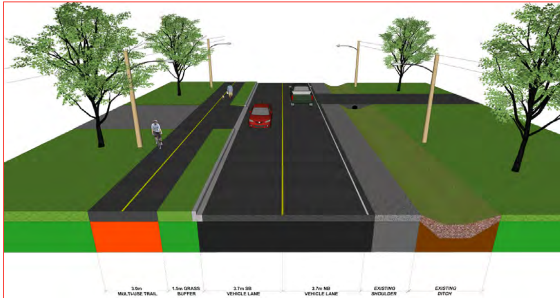
Figure 6-1: Proposed Lucasville Road Cross Section with curb looking north
