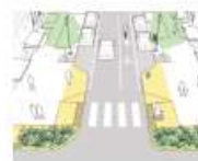
Curb Extensions aka Bump-Outs (reduce speed, crossing distance)
