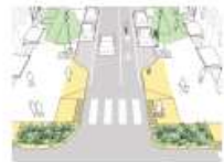
Curb Extensions aka Bump-Outs (reduce speed, crossing distance)
