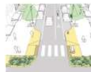
Curb Extensions aka Bump-Outs (reduce speed, crossing distance)
