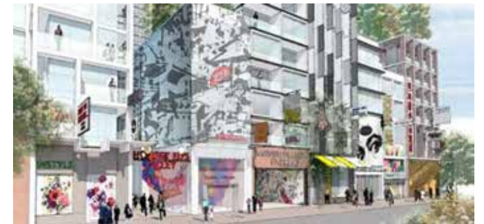
Highly articulated lower floors with frequent entrances, varying setbacks and street-faces of 2-6 storeys (Images: Mirvish Village, Toronto)
